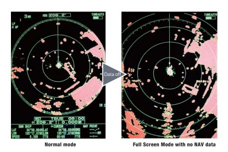
There is also an option to clear the navigation data on the Radar display. Individual navigation data can be easily toggled ON or OFF in the dedicated menu.
