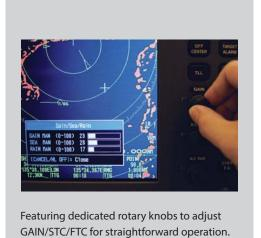
Rain disturbs target recognition on the Radar screen.
